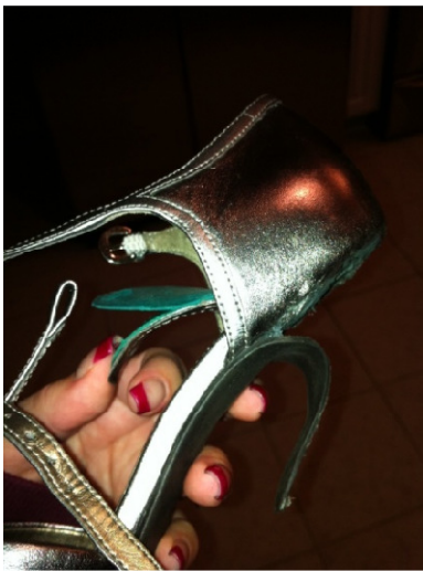
Figure 56: Naturalizer brand high heel with sole uplifted and heel removed so that the twist and lock heel can be attached.
